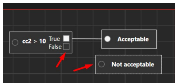
Figure 7.163 Conditional node with connected "Acceptable" result node
